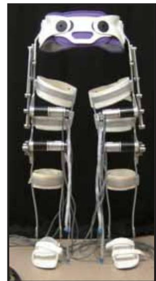
Fig.1 Powered assistive orthosis
