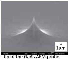
tip of the GaAs AFM probe
