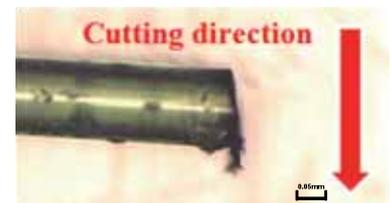
Fig. 8 Cross-sectional microscopic image of the artificial hair cut by rotary type shaver
