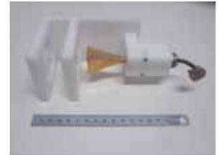
Fig.2 The focusing lens sensor
