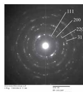
Fig.5 Diffraction patterns image of Au nanowire.
